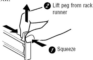
Re-insert the rack in the chosen position and replace the pegs. Check that the spray arm is free to rotate.
