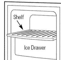
Pull the upper freezer shelf straight out to access the icemaker. Always be sure to replace the shelf. The shelf can be used for storage.
