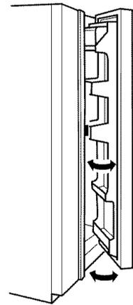
When the door is only partially open, it will automatically close.
