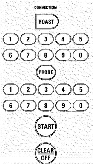
To change the oven temperature during the Convection Roast cycle, touch the **CONVECTION ROAST** pad and then touch the number pads to set the new desired temperature.
