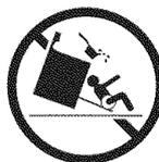
**⚠ WARNING** To reduce the risk of tipping, the range must be secured by properly installed anti-tip bracket provided with the range. To check if the bracket is installed properly, grasp the top rear edge of the range and carefully attempt to tilt it forward. Refer to the Installation Instructions for proper anti-tip bracket installation.
