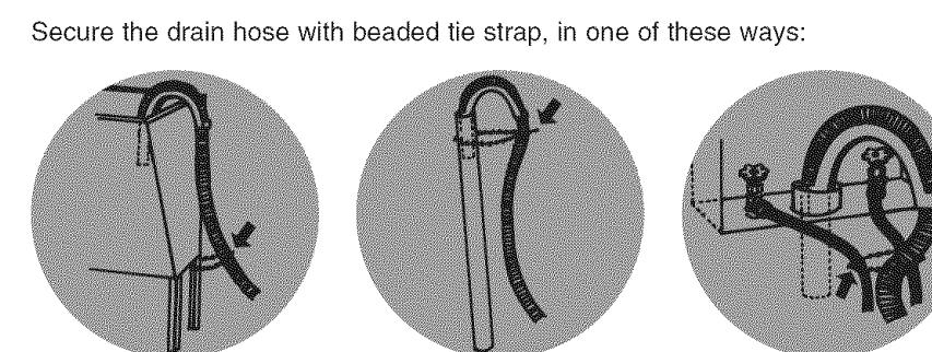
Secure the drain hose with beaded tie strap, in one of these ways:
