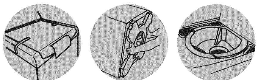
Lid must be taped in place prior to moving the washer.
