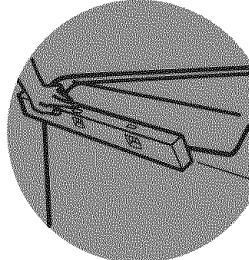
Push on the upper front panel to be sure that the washer is on the rear feet. Lower right front foot to floor. By hand, firmly rotate foot up an additional ½ turns. Rock washer gently front to back, side to side and diagonally to check that all four feet are in firm contact with the floor.
