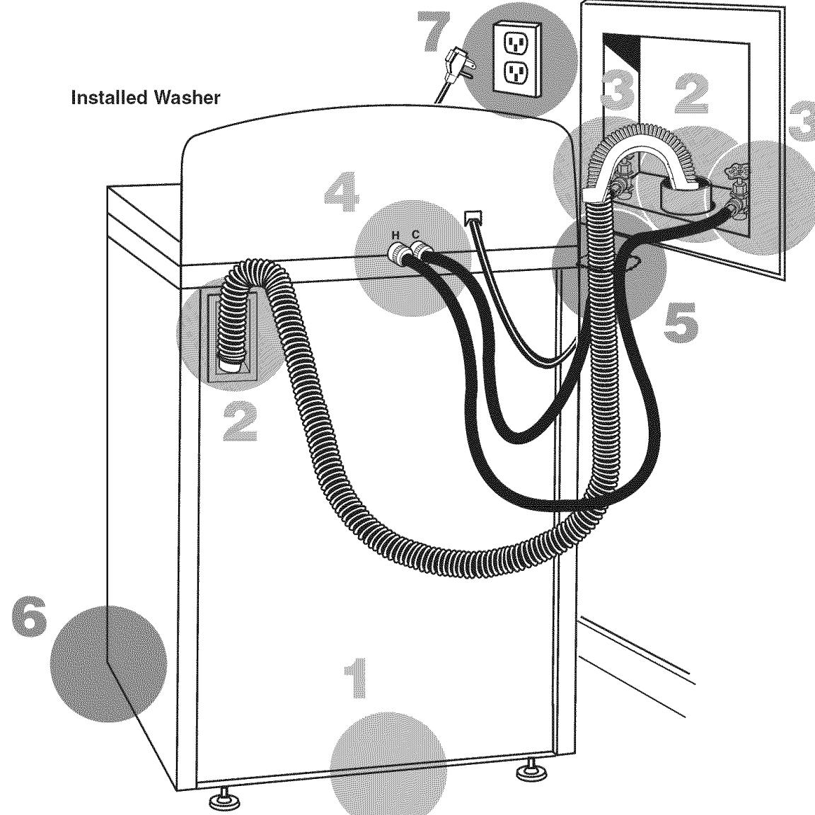
Move washer to its final location and level the washer.
