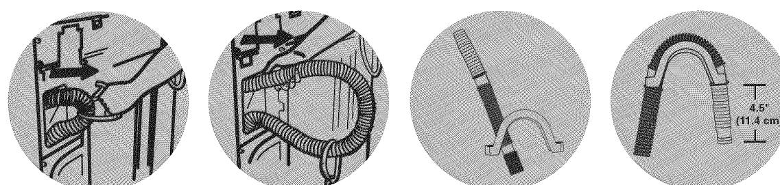
Locate the pull tie to remove drain hose from washer. Pull drain hose straight out of washer from top of hose. Continue to pull the hose until the end emerges.
