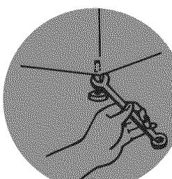
Check levelness on both the front and side of the washer.
