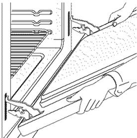
HINGE SLOT - Door removed
