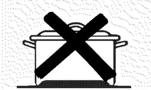
Pans with rounded, curved, ridged or warped bottoms are not recommended.
