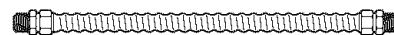
CSA-Approved Flexible Gas Line 3/8" Min. ID, 1/2" NPT Connection, 3-foot Maximum Length (Massachusetts Only)
