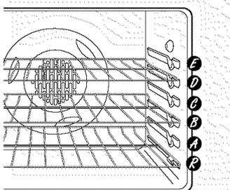
When convection baking with only 1 shelf, follow the shelf positions recommended in the Using the Oven section.
