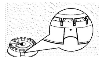
Use a sewing needle or twist-tie to unclog the small hole in the burner head.
