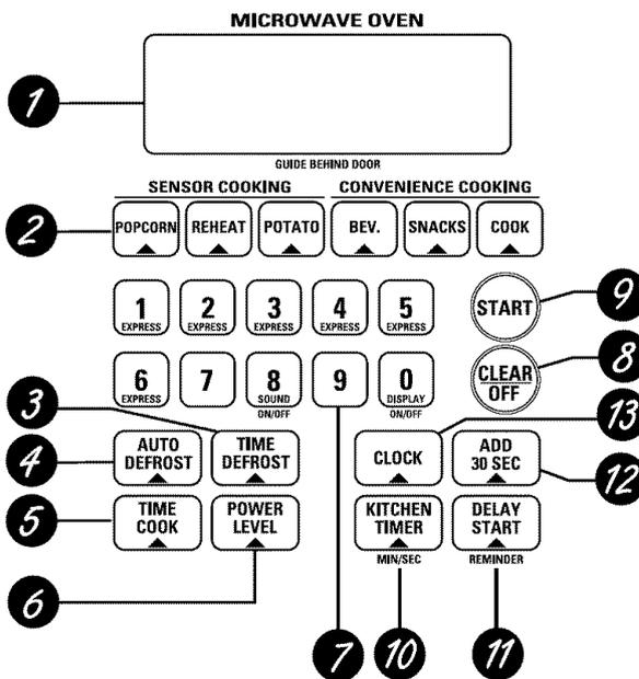
The time on the microwave display is shown in minutes and seconds (1:30 is one minute, 30 seconds). On the lower oven, time is shown in hours and minutes (1:30 is one hour, 30 minutes).
