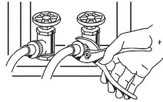
**NOTE:** Do not overtighten or use tape or sealants on the valve. Damage to the valves can result.
