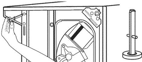
2. Check adjustability of rear legs by pushing in one leg. The other leg should come out. Check both legs. If they do not move freely, repeat Step 1.
