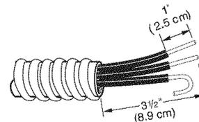
When connecting to the terminal block, place the hooked end of the wire under the screw of the terminal block (hook facing right), squeeze hooked end together and tighten screw.
