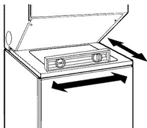
2. If the washer/dryer is not level, prop up the front with a wood block and adjust the feet up or down as necessary. Remove wood block and lower washer/dryer. Repeat this step until the washer/dryer is level.
