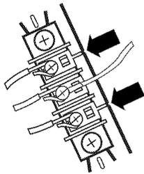
5. Tighten strain relief screw.
