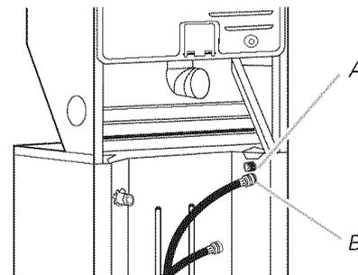
A. Cold water inlet valve (top)
