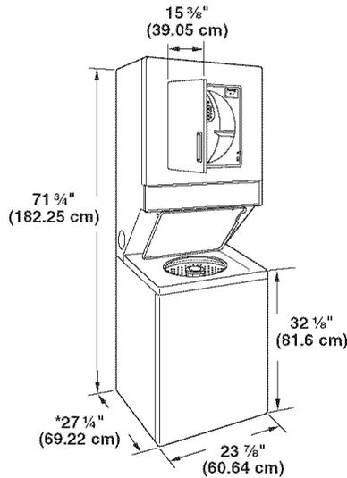
\*Most installations require a minimum 5 1/2" (14 cm) clearance behind the dryer for the exhaust vent with elbow. See "Venting Requirements."
