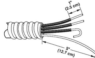
When connecting to the terminal block, place the hooked end of the wire under the screw of the terminal block (hook facing right), squeeze hooked end together and tighten screw. See example below.
