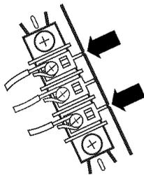
4. Tighten strain relief screw.
