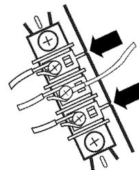
4. Tighten strain relief screws.
