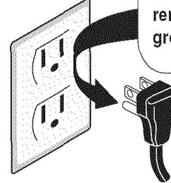
Power supply cord with 3-prong grounding plug
