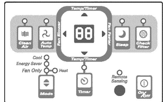
A 2 Digit Display is used to indicate the Fan Speed setting, from 10 through 99. When the “SLOWER” button is pressed the motor speed will slow down at various intervals, down to a minimum setting of 10. To speed the motor up, press the “FASTER” button. The speed will increase at multiple intervals to a maximum setting of 99. Display will revert back to temperature setting after a short time.
