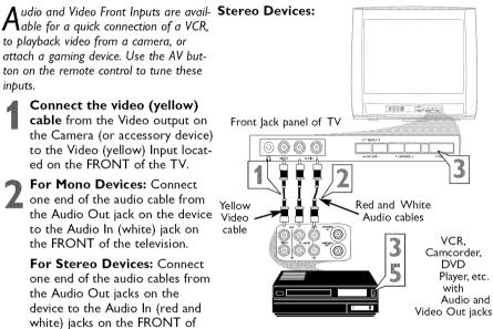
to playback video from a camera, or attach a gaming device. Use the AV button on the remote control to tune these inputs.
