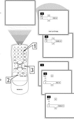
Press SURF repeatedly during TV viewing to scan through the channels in the SURF list.
