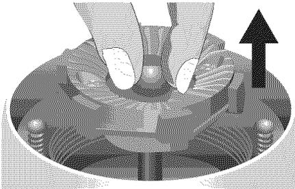
5. Lift the burr-shaft assembly out of the motor housing.
