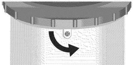
3. Using a Phillips-head screwdriver, turn the set screw counter-clockwise to loosen, and remove.
