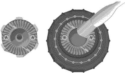
**NOTE:** Never wash the burrs or burr-shaft assembly in water. Keep them dry at all times.
