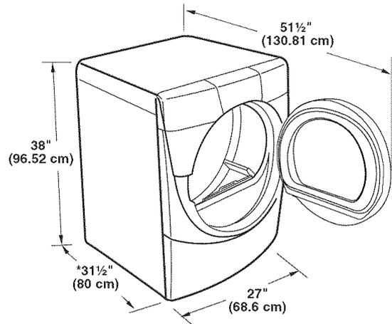
\*Most installations require a minimum 5½" (14 cm) clearance behind the dryer for the exhaust vent with elbow. See "Venting Requirements."
