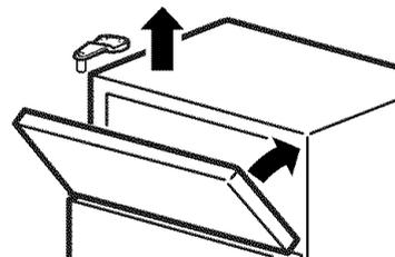
6.2.3. Make sure the door is slightly above the top of the cabinet and the gap between the doors is even across the front. Tighten the top hinge screws. Do not overtighten these screws—tighten them until they are just snug, then turn them another one-half turn.
