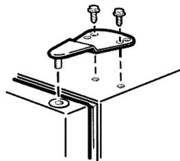
Installing the hinge on the left. Installing the hinge on the right.
