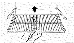
**To remove a full-width shelf when the fresh food compartment door cannot be opened fully,** lift the rear of the shelf, pull forward and down, tilt the shelf and take it out.
