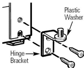
Models with a hinge bracket that has 2 screw holes.
