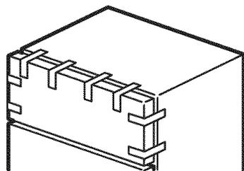
2.2 With a 5/16" hex-head socket driver, remove the screws that hold the top hinge to the cabinet.
