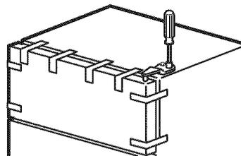
2.3 Lift the hinge (and the shim glued to it) straight up to free the hinge pin from the socket in the top of the door and set it aside, along with its screws.
