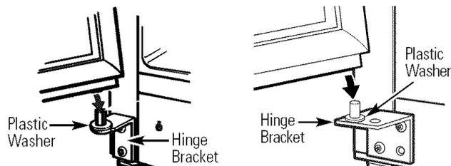
Models with a hinge bracket that has 2 screw holes.
