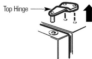
2.4 Remove the tape and tilt the door away from the cabinet. Lift it off the center hinge pin.
