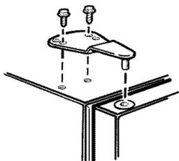
Installing the hinge on the left.
