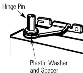
5.2.2 Tilt the door toward the cabinet, lifting the top hinge so the pin fits into the socket on the top of the door.
