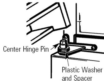
5.1.2 Insert the pin on the center hinge into the socket in the top of the door. Place the spacer, then the washer, on the hinge pin. **NOTE:** The center hinge must be turned over as shown when mounted on the left side.
