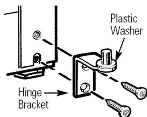
Models with a hinge bracket that has 2 screw holes.
