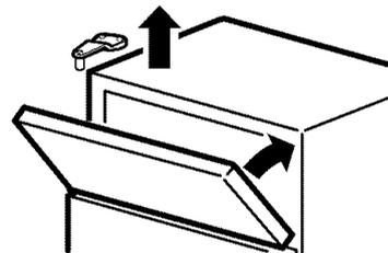
5.1.3 Tilt the door toward the cabinet. As the door is brought into position, slide the hinge under the head of the screw which earlier had been partly driven into the outermost hole. Insert the remaining screw, then tighten both screws securely.
