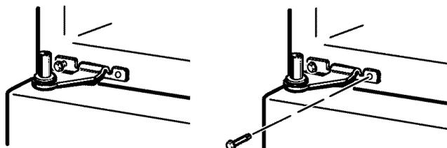
5.2.3 Make sure the door is slightly above the top of the cabinet and the gap between the doors is even across the front. Tighten the top hinge screws. Do not overtighten these screws—tighten them until they are just snug, then turn them another one-half turn.
