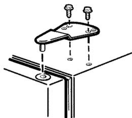
Installing the hinge on the right.
