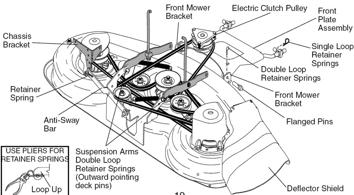
**NOTE:** To assist in locating hole in flanged pin, the hole in pin is inline with notch on head of pin. If necessary, move mower side-to-side to give space between plate and mower brackets.
