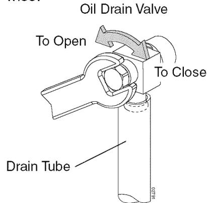
4. After oil has drained completely, close the drain valve turning completely clockwise. Use the 7/16" (11mm) wrench to apply a small amount of torque to keep it closed. Do not over tighten.
