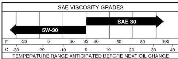
**NOTE:** Although multi-viscosity oils (5W30, 10W30 etc.) improve starting in cold weather, they will result in increased oil consumption when used above 32°F. Check your engine oil level more frequently to avoid possible engine damage from running low on oil.
