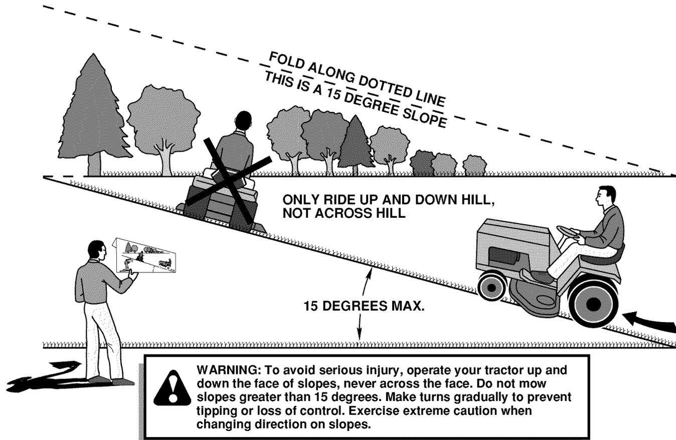
**WARNING:** To avoid serious injury, operate your tractor up and down the face of slopes, never across the face. Do not mow slopes greater than 15 degrees. Make turns gradually to prevent tipping or loss of control. Exercise extreme caution when changing direction on slopes.
