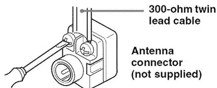
**1** Loosen the screws on the antenna connector.
