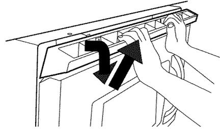
3. Slide filter back slightly, lift front end, and pull out filter.
