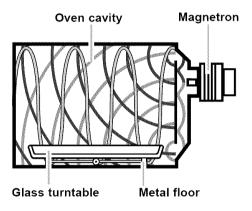
The glass turntable of your microwave oven lets microwaves pass through. Then they bounce off a metal floor, back through the glass turntable, and are absorbed by the food.
