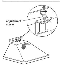
Align the "T" area of the canopy hood slots with the lower bracket flanges. Push hood toward wall. Gently lower the hood making sure the lower bracket flanges are fully inserted into the slots. Check that the hood is secure on the lower bracket. Feed enough power supply cable through conduit connector to make electrical connections.
