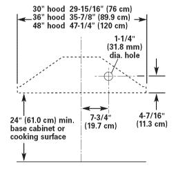
Determine the required height for the power supply cable and cut a 1-1/4" (3.2 cm) hole at this location. Run wire through hole according the National Electrical Code or CSA Standards and local codes and ordinances. There must be enough power supply cable from the fused disconnect (or circuit breaker) box to make the connection in the hood's electrical box.
