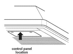
18. The canopy hood controls are located in a grey panel on underside of the canopy. To open the panel, press on the front edge of panel and release. The control panel will drop down.
