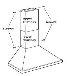
15. When upper and lower chimney sections are in final position, attach the top of the upper chimney and the bottom of the lower chimney to the top and bottom brackets.
