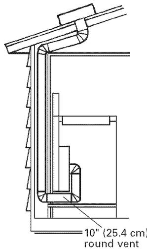
It is recommended that you use round vent instead of rectangular vent, especially if elbows are required. If rectangular vent is required, it should be transitioned to 10" (25.4 cm) round vent as soon as possible.
