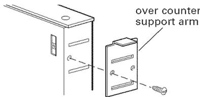
**2.** Attach the left side and right side overcounter support brackets to the downdraft. Use 1 screw with each bracket.
