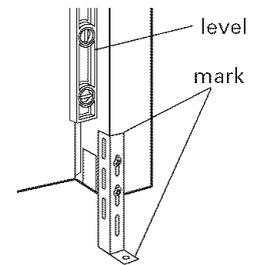
**6.** Move support legs down against cabinet floor. Place a level against front of downdraft vent base and adjust until downdraft vent is level vertically. Use a pencil to mark the top of each leg on downdraft vent. Then mark location of support leg mounting holes on cabinet floor. Remove downdraft vent from cutout. Drill starter holes at each mounting screw location on cabinet floor. Align top of legs with pencil marks on the face of the downdraft vent. Tighten screws in legs.
