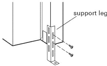
**4.** Attach support legs to side of downdraft vent with two screws in each leg. Do not tighten screws.
