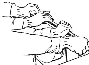
**5.** Carefully insert downdraft vent into countertop cutout. Two people are recommended to support the weight of the downdraft vent during lifting. Check that downdraft vent is parallel to side of cutout and that mounting brackets overlap countertop.
