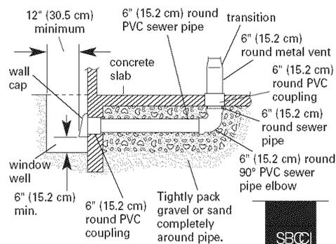
Seal the space between the outside of wall cap inlet inside of PVC coupling with caulking metal.
