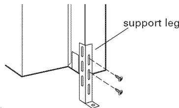
**4.** Attach support legs to side of downdraft vent with 2 screws in each leg. Do not tighten screws.
