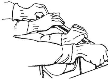
**5.** Carefully insert downdraft vent into countertop cutout. Two people are recommended to support the weight of the downdraft vent during lifting. Check that downdraft vent is parallel to side of cutout and that mounting brackets rest gently on countertop.
