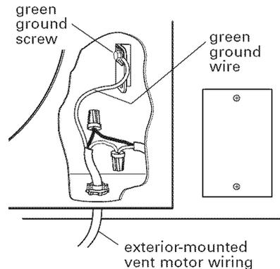
**14.** Remove vent box knockout and install conduit connector. Feed exterior-mounted vent motor wiring through conduit connector.
