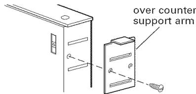
**2.** Attach the left side and right side overcounter support brackets to the downdraft. Use 1 screw with each bracket.
