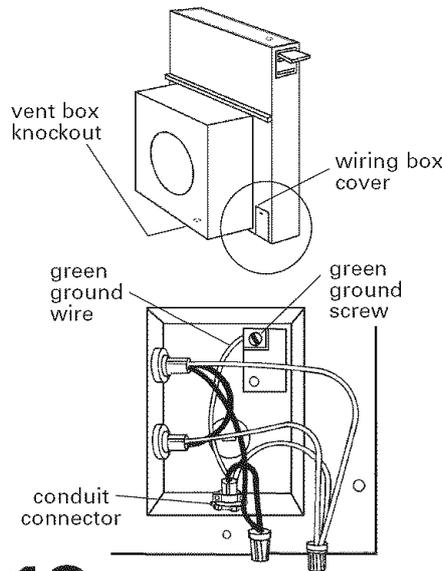
**13.** Feed the power supply cable through the conduit connector and into wiring box. Connect the white wires together with a twist-on wire connector. Connect the black wires together with a twist-on wire connector. Attach the green (or green and yellow) ground wire to eyelet with green ground screw and tighten screw. Replace wiring box cover.
