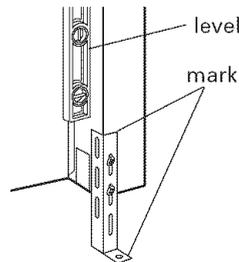
**6.** Move support legs down against cabinet floor. Place a level against front of downdraft vent base and adjust position of legs until downdraft is level vertically. Use a pencil to mark the top of each leg on face of downdraft vent. Then mark location of support leg mounting holes on cabinet floor. Remove downdraft vent from cutout. Drill starter holes at each mounting screw location on
