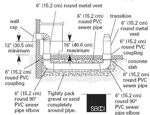
Optional vent system installed under a concrete slab into a window well.
