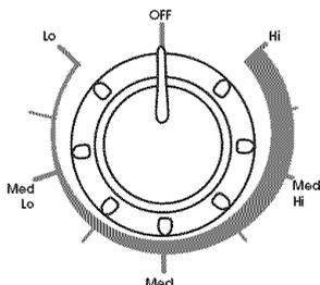
Push in and turn to the desired heat setting. Use the following chart as a guide when setting heat levels.
