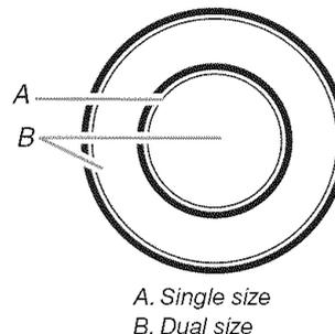
The Dual-Size Elements offer flexibility depending on the size of the cookware. Single size can be used in the same way as a regular element. The dual size combines both the single and outer element and is recommended for larger size cookware, large quantities of food and home canning.
