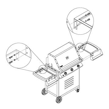
Step 9: Attach and secure the condiment tray to control panel with 1 piece crossed round head screw (5/32" x 8mm) & washer.
