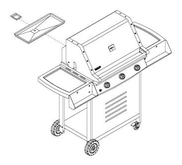
STEP 11: Place L.P tank in tank seat hole and secure with retention wing-bolt.
