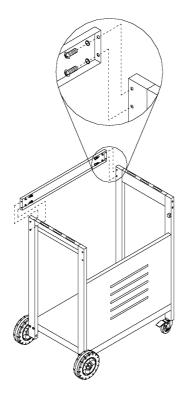
STEP 5: Remove grill head unit from carton. Place onto cart from above as shown on diagram (below). And secure to cart frame.
