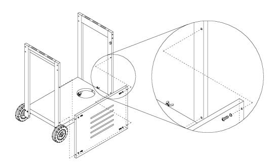
STEP 4: Attached and secure the cart frame crossed bar to the top back of both side panels by using 4 pieces (1/4" x 10 mm) crossed round head screws & washers.
