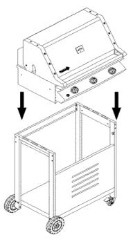
STEP 6: Secure the head unit to cart with 4 pieces crossed round head screws (1/4" x 15mm) and flat washers as shown on diagram below. (Note: Remove cooking grids and flame tamers before this step)
