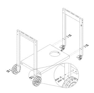
STEP 3: Assemble front panel to side panel legs with 4 pieces crossed round head screws (1/4" x 10mm) and washers as shown figure below.
