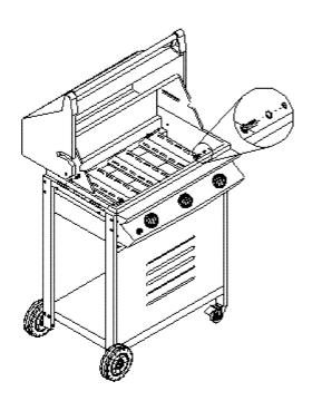
STEP 7: Attach and secure the nip clip and the regulator hose to the right panel leg with 1 piece crossed round head screw (1/4"x10) and washer as below shown.
