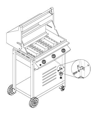
STEP 8:Attach left side shelf with 4 pieces crossed round head screws (1/4" x 10mm) and washers as shown on below figure.
