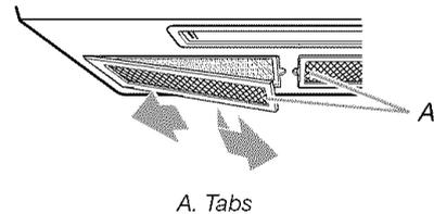
2. Remove charcoal filters by pushing the back of each filter away from you until the front of the filter slides off the front lower lip. Swing the front of the filter down and slide out.
