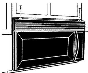
3. Tip the grille forward, then lift out to remove.
