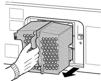
**NOTE:** Wear soft, lint-free gloves when replacing the lamp unit.
