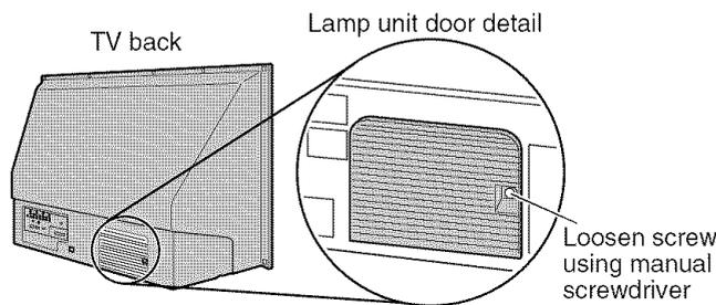
**4** Using a manual Phillips screwdriver, loosen the two screws on the lamp unit.
