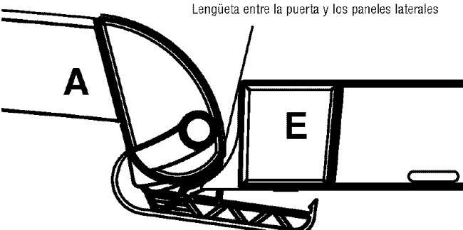
20. Place the door hook tab between the Door Panel (A) and the Side Panel (E) as shown in the view to the left.
