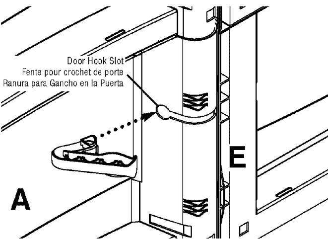
19. Guide Door Hook (P) along the door hook slot, moving snap end of the Door Hook (P) towards Side Panel (E).
