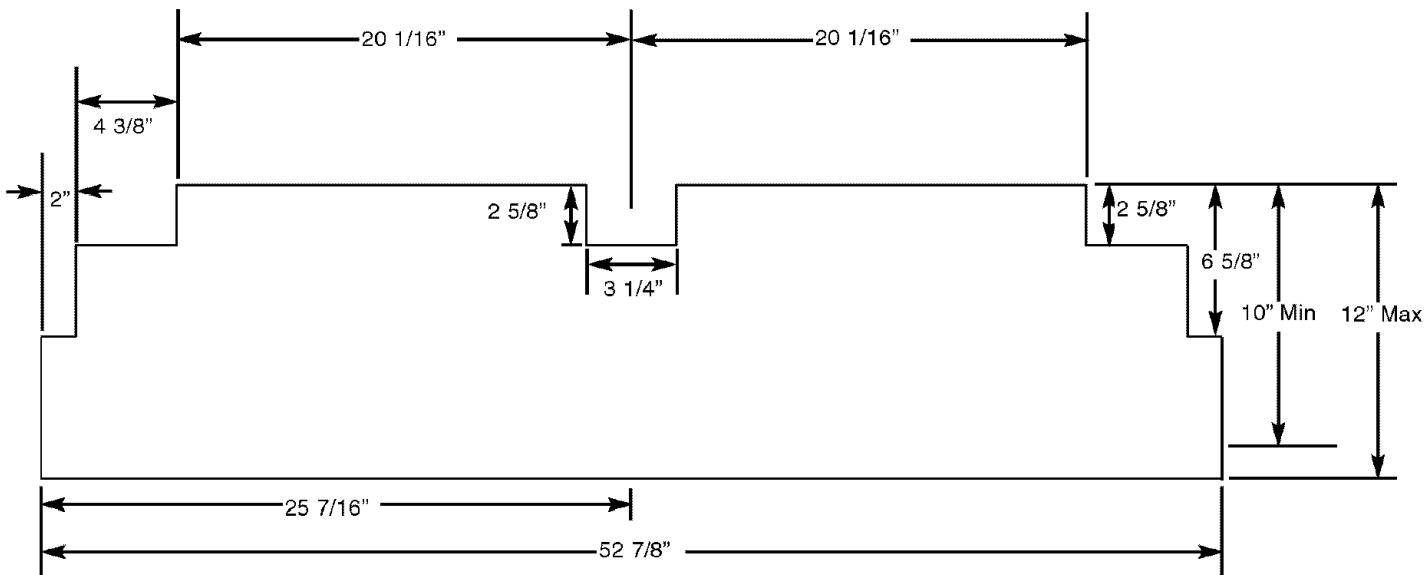
**Shelving:** Shelving can be added to your Suncast storage shed by utilizing the provided dimensions and cutting your own shelf from 1" thick shelving material. The notched corners face the back of the shed and fit into the inner shelf brackets that have been molded into the inner sides of your storage shed.
