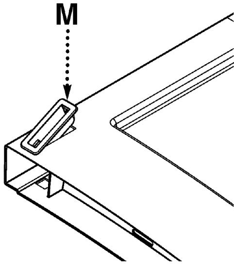
9. Locate door latch assembly housing receptacle in the lower right door. Insert Door Latch Housing (M) into door latch receptacle.
