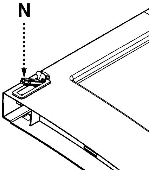
10. Insert the Door Latch Pin (N) into the Door Latch Housing. Push Door Latch Pin downward to engage snaps that secure it in housing.
