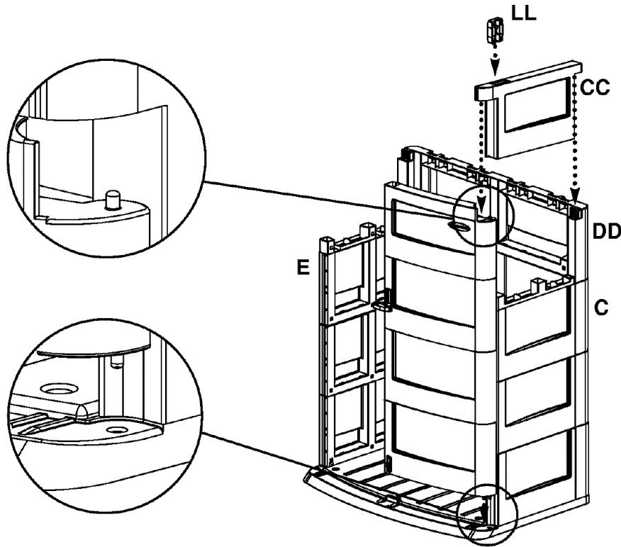
13. Place Upper Right Side Top Connector (LL) in upper right side cap receptacle located in the Upper Right Side Panel (CC). Press down until Upper Right Side Cap snaps into place.
