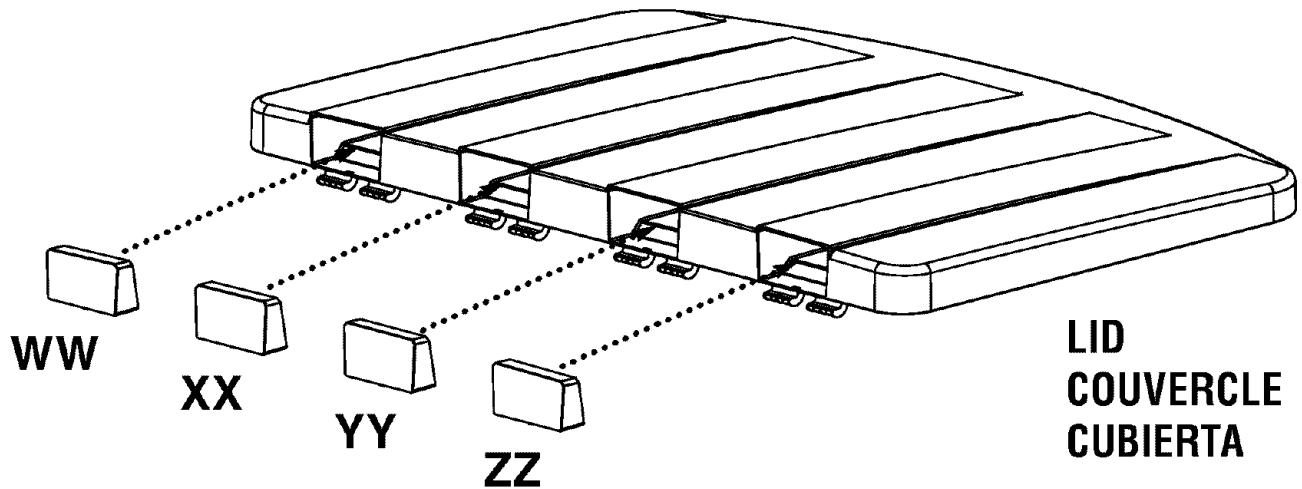
22. Assemble Lid by taking Lid End Caps (WW, XX, YY, ZZ) and pushing them into the respectively marked openings in the Lid.
