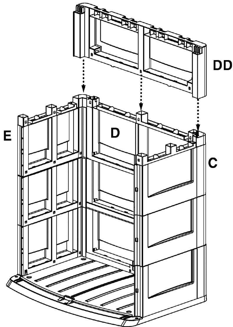
12. Place Upper Back (DD) onto Lower Back (D) making sure to connect to Lower Sides (E,C). Press down until Upper Back snaps into place.
