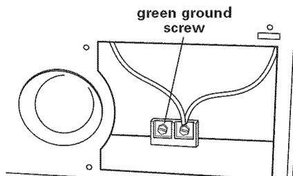
**21.** Connect the white and black wires of power supply cable to the white and black leads in hood with twist-on connectors.
