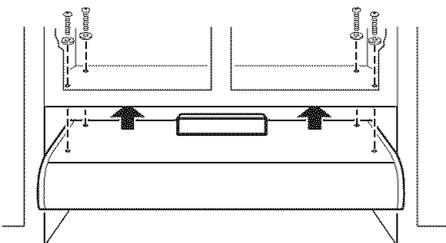
**19.** Lift hood into place while feeding wiring into wiring box.
