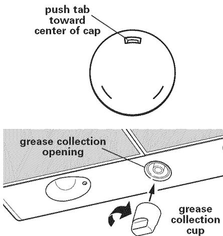
**25.** Remove plastic cap located between lights. Locate tab in cap's large slot. Use a small flat-bladed screwdriver and press tab toward center of cap to release tab. Squeeze cap to release other 2 tabs and discard cap.
