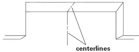
**5.** Mark centerlines on rear wall and upper cabinet bottom.
