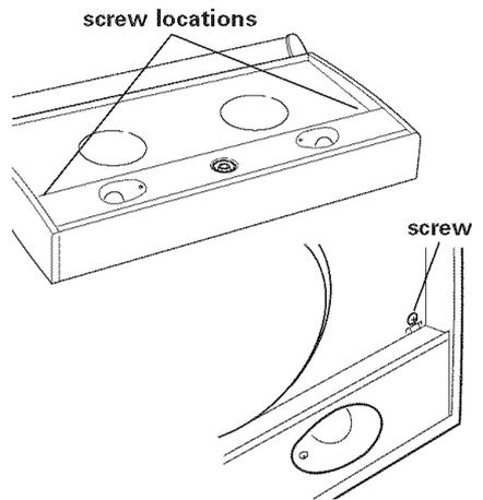
**14.** Remove 2 screws from light panel tabs. On light panel surface directly behind tabs, push toward back of the hood to move tabs out through the slots. Remove panel and set aside with screws.
