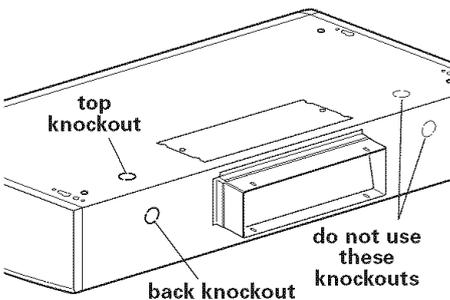
**4.** Remove knockout from the wiring opening (top or back) to be used.
