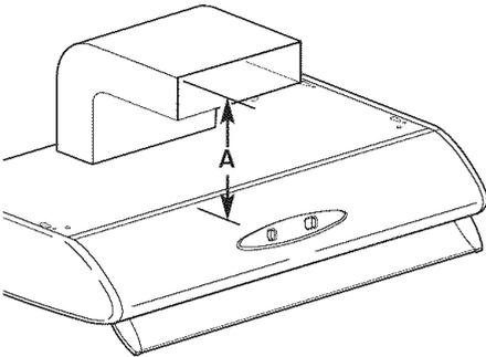
Measure distance A and transfer it to the centerline on the soffit. Mark and cut a 3-1/4" x 10" (8.3 cm x 25 cm) vent opening in the soffit.
