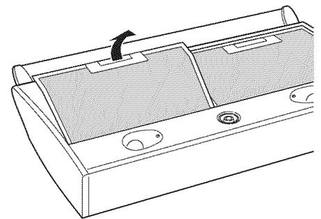
**13.** Rotate deflector away from filters. Pull grease filter handles toward back of hood to release locking tabs. Lift filters up, remove from hood and set aside.
