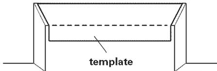
**6.** Align centerlines of template with centerlines marked on rear wall and upper cabinet bottom. Tape template in place. Mark location of the four holes used to secure hood to upper cabinet.
