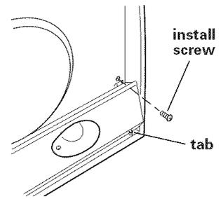
**22.** Reinstall light panel. Insert light panel tabs into slots. Push in on back of light panel and insert the small tabs into the locating holes in back of the hood. Reinstall the 2 screws and tighten securely.
