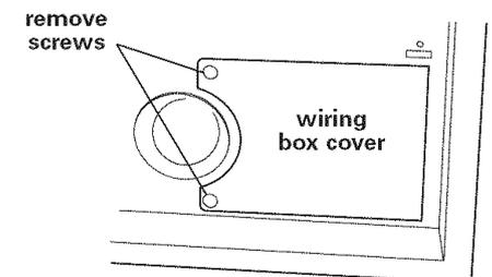
**15.** Remove 2 screws from wiring box cover located in the right hand rear corner and remove cover. Attach the U.L.- or CSA-listed strain relief to the hood wiring hole being used.
