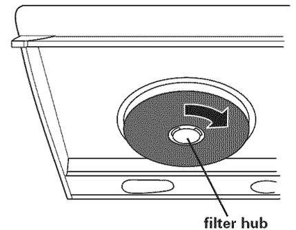
**23. Non-vented (recirculating) installations:** Install the charcoal filters. Place filter over hub in blower openings, push up and turn clockwise to lock filter into place.
