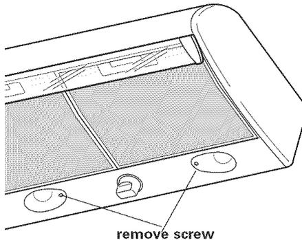
**Replacing lights:** Use a Phillips screwdriver to remove screw holding the light
