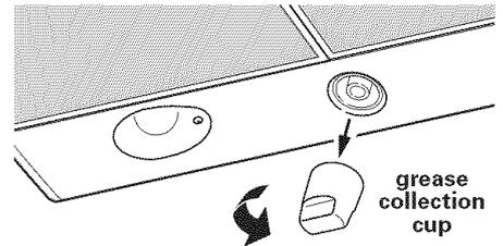
**Cleaning grease collection cup:** Twist cup counterclockwise to remove. Wash in hot sudsy water. Dry, insert into opening and twist clockwise.
