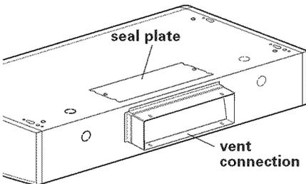
**If venting through the wall,** remove seal plate from back of hood and vent connector from top of hood. Reinstall vent connector on back of hood and seal plate on top of hood.
