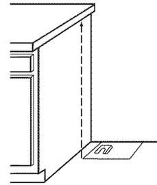
If cabinet opening is wider than specified in the "Location Requirements" section, adjust template so range will be centered in cabinet opening.
