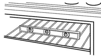
If range is not level, pull range forward until rear leveling leg is removed from the anti-tip bracket. Use  $\frac{3}{8}$ " drive ratchet and channel lock pliers to adjust leveling legs up or down until range is level. Push range back into position. Check that rear leveling leg is engaged in anti-tip bracket.
