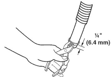
4. Open clamp. Twist hose back and forth while pushing onto drain connector on the side of the washer/dryer. Continue until hose contacts the ribbed stops on the cabinet.
