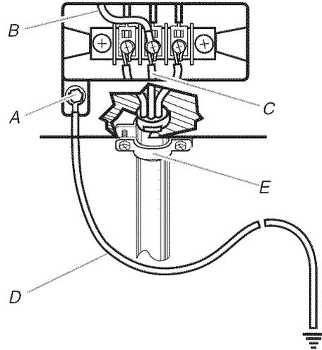
A. External ground conductor screw
