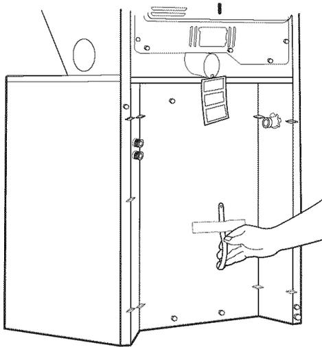
2. Tilt the washer/dryer forward. Move each of the 2 rear legs in an up-down motion to check the self-adjusting leveling legs for free movement. This is required for proper leveling. Gently lower the washer/dryer to the floor.
