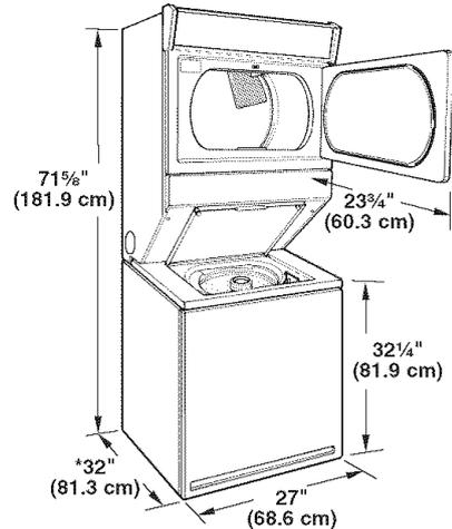
\*Most installations require a minimum 5 1/2" (14 cm) clearance behind the dryer for the exhaust vent with elbow. See "Venting Requirements."
