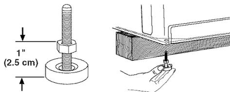
3. Screw the feet into the correct holes at the front corner of the washer/dryer until the nuts touch the washer.
