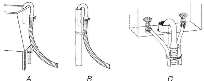
If the water faucets and the drain standpipe are recessed, put the hooked end of the drain hose in the standpipe. Tightly wrap the shipping strap around the water inlet hoses and the drain hose (C above). Push fastener into the nearest hole in the shipping strap (see illustration above).
