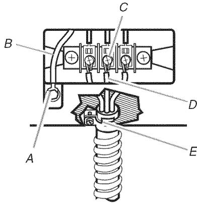
A. External ground conductor screw
