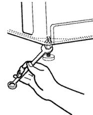
3. Tilt the washer/dryer forward until the rear of the washer/dryer is at least 4" (10.2 cm) off the floor. You may hear the self-adjusting rear feet click into place. Lower the washer/dryer to the floor. Check the levelness of the washer/dryer with a level as shown above.
