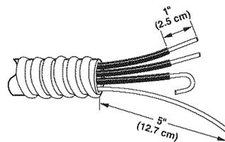
When connecting to the terminal block, place the hooked end of the wire under the screw of the terminal block (hook facing right), squeeze hooked end together and tighten screw, as shown.
