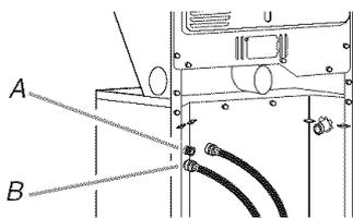
A. Cold water inlet valve (top)
