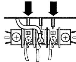
4. Tighten strain relief screws.
