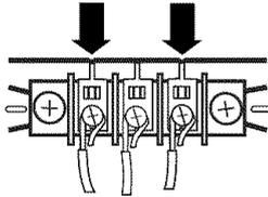
4. Tighten strain relief screw.
