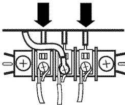
5. Tighten strain relief screw.
