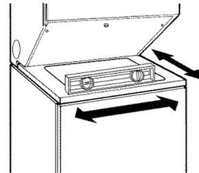
2. If the washer/dryer is not level, prop up the front with the wood block and adjust the feet up or down as necessary. Remove wood block.
