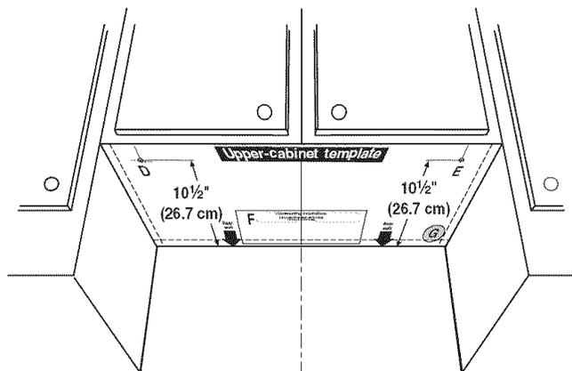
5. Cut the 1½" (3.8 cm) diameter hole at the circular shaded area "G" on the template. This hole is for the power supply cord.
