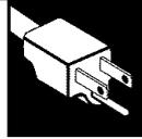
This appliance must be grounded. In the event of an electrical short circuit, grounding reduces the risk of electric shock by providing an escape wire for the electric current. This appliance is equipped with a power cord having a grounding wire with a grounding plug. The plug must be plugged into an outlet that is properly installed and grounded. (Fig. 1)
