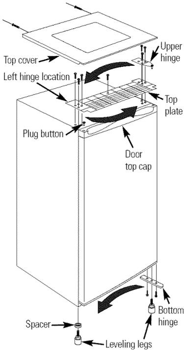
1. Remove the two screws at the back of the top cover.
