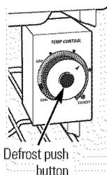
Defrosting usually takes a few hours. When defrosting is complete, the red "Defrost Button" will release automatically. Then the refrigerator will resume normal operation while moving towards the set temperature. **NOTE:** After defrosting, allow a few hours to reach the set temperature before making any further adjustments.
