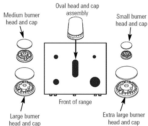
Place the burner caps on the cooktop. Make sure that the caps are placed in the correct locations. There is one oval (center) head and cap assembly, one small cap, one medium cap, one large cap, and one extra large cap.
