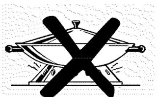
Do not use a wok support ring. Placing the ring over the burner or grate may cause the burner to work improperly, resulting in carbon monoxide levels above allowable standards. This could be dangerous to your health.
