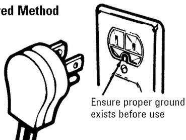
The power cord of this appliance is equipped with a three-prong (grounding) plug which mates with a standard three-prong grounding wall receptacle to minimize the possibility of electric shock hazard from this appliance.
