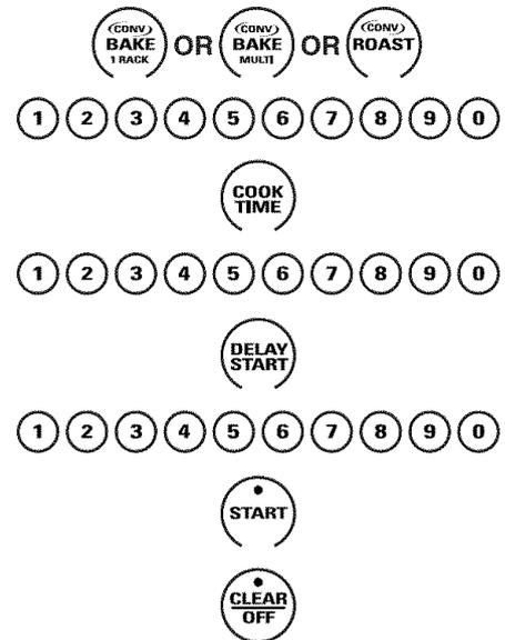
The oven will continue to cook for the programmed amount of time, then shut off automatically, unless the WARM feature was set. See the *How to set the oven for warming* section.
