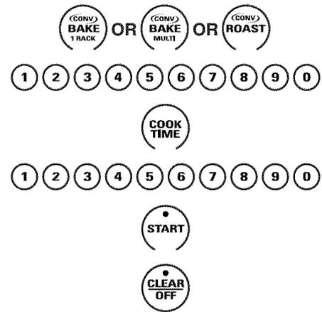
The oven will continue to cook for the programmed amount of time, then shut off automatically, unless the WARM feature was set. See the *How to set the oven for warming* section.
