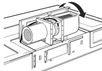
6. Tilt and place the blower unit back into the opening in the top of the microwave.
