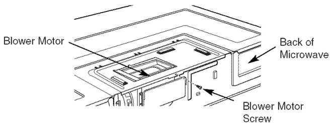
2. Open the blower motor door by lifting it up at the back side of the microwave. Remove and save the top and back retaining screws that hold the blower motor in the microwave.
