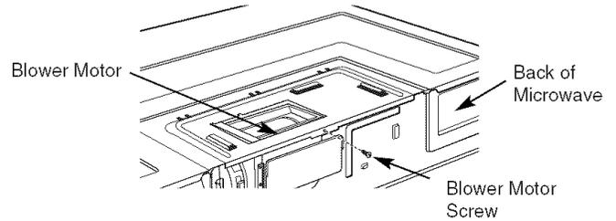
2. Open the blower motor by lifting it up at the back side of the microwave. Remove and save the top and back retaining screws that hold the blower motor in the microwave.
