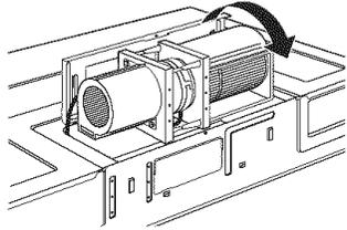
6. Tilt and place the blower unit back into the opening in the top of the microwave.
