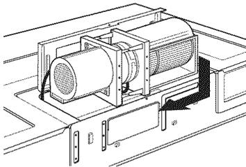
7. Secure the blower unit to the microwave with the two screws removed in Step 2.
