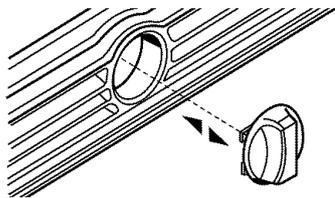
3. Rotate the cartridge cap to a horizontal position.
