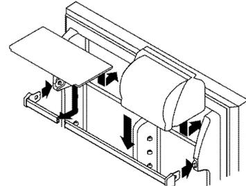
3. Adjust the utility compartment by lifting the front slightly and sliding it to the desired position. Lower the front to lock it into place.
