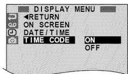
\* Each setting is linked with "DISPLAY MENU", which appears when the Power Switch is set to "M" (pg. 27). The parameters are the same as in the description on page 27.
