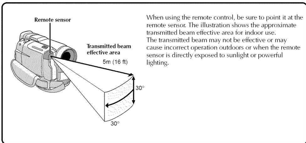
When using the remote control, be sure to point it at the remote sensor. The illustration shows the approximate transmitted beam effective area for indoor use. The transmitted beam may not be effective or may cause incorrect operation outdoors or when the remote sensor is directly exposed to sunlight or powerful lighting.
