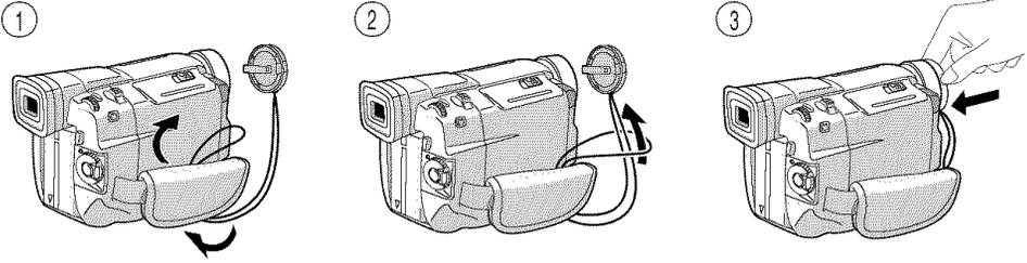
To protect the lens, attach the provided lens cap to the camcorder as shown in the illustration.
