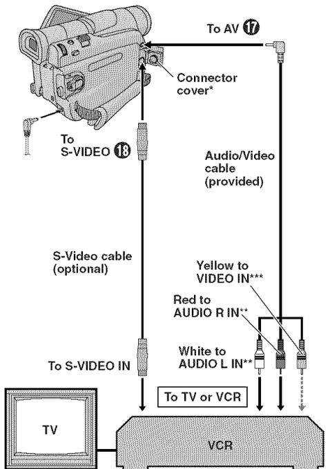
\* When connecting the cable, open this cover.
