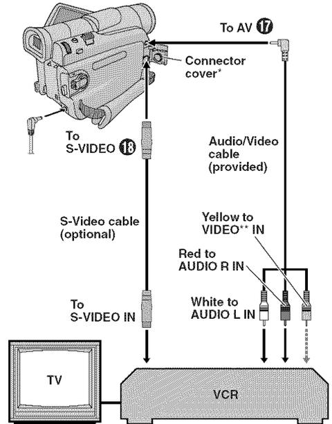
\* When connecting the cable, open this cover.
