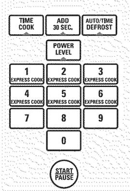
Variable power levels add flexibility to microwave cooking. The power levels on the microwave oven can be compared to the surface units on a range. High (power level 10) or full power is the fastest way to cook and gives you 100% power. Each power level gives you microwave energy a certain percent of the time. Power level 7 is microwave energy 70% of the time. Power level 3 is energy 30% of the time.
