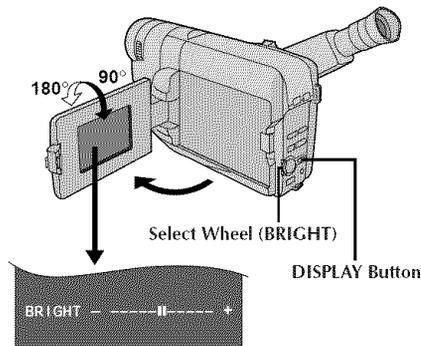
**To Adjust The Brightness Of The LCD Monitor**
