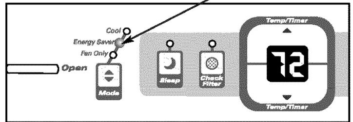
Note: In this mode, the fan will continue to run for 3 minutes after the compressor shuts off. The fan then cycles on for 2 minutes at 10 minute intervals until the room temperature is above the set temperature, at which time the unit turns back on.
