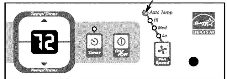
Note: Fan speed starts at high and adjusts to a slower speed as the room temperature dictates. For example, if the room doesn't get too warm it will stay at the slowest speed. If the room temperature rises quickly, such as a door being opened, it will automatically go to the highest speed. The fan speeds will readjust back to the slowest speed as the room returns to the original set temperature. Press the Fan Speed button to adjust the fan speed manually.
