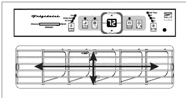
The 4-Way air directional louvers allow you to direct air flow up or down, left or right throughout the room as needed.
