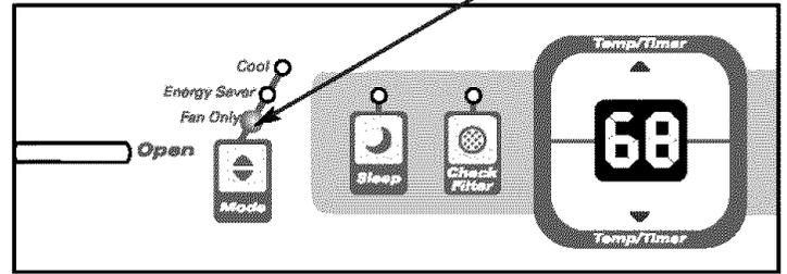
Note: Use this function only when cooling is not desired, such as for room air circulation or to exhaust stale air (Remember to open the vent during this function, but keep it closed during cooling for maximum cooling efficiency). You can choose any fan speed you prefer. During this function, the display will show the actual room temperature, not the set temperature as in the cooling mode.
