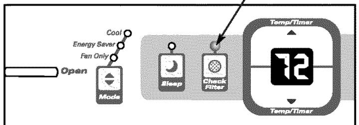
Note: This feature is a reminder to clean the Air Filter (See Care and Cleaning) for more efficient operation and cooling. The LED (light) will illuminate after 250 hours of operation. To reset after cleaning the filter, press the “ Check Filter ” button and the light will go off.
