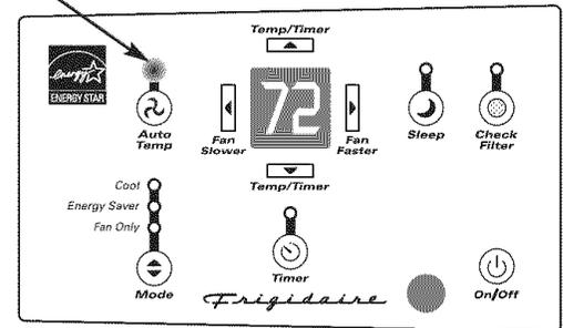
**Note:** Fan speed starts at High Speed and adjusts to a slower speed as the room temperature dictates. For example if the room doesn't get too warm, it will stay at the slowest speed. If the room temperature rises quickly, such as a door being opened, it will automatically go to the highest speed. The fan speeds will re-adjust back to the slowest speed as the room returns to the original set temperature.
