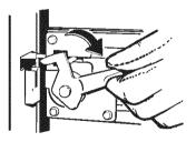
Hold the side door latch and tilt the side of the drawer until the latch clears the drawer front. The drawer side can be removed by tilting and sliding it out.
