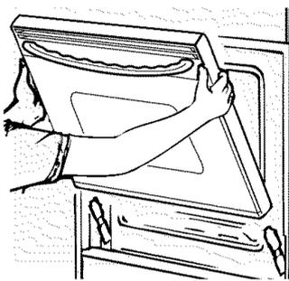
The oven door is removable for easier access to the light bulb. Lift the door straight up and off the hinges. Do not lift the door by the handle.
