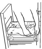
**3.** Push the side-lock latch down and tilt the drawer side open.
