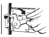
**3.** Hold the side door latch and tilt the side of the drawer until the latch clears the drawer front. The drawer side can be removed by tilting and sliding it out.
