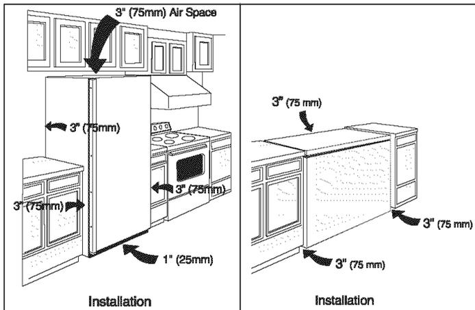
**NOTE:** The exterior walls of the freezer may become quite warm as the compressor works to transfer heat from the inside. Temperatures as much as 30° F warmer than room temperature can be expected. For this reason it is particularly important in hotter climates to allow enough space for air circulation around your freezer.
