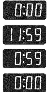
**Note:** The minute timer does not start or stop cooking. It serves as an extra timer in the kitchen that will beep when the set time has run out. The minute timer can be used alone or during any of the other oven functions. When the minute timer is in use with any other mode, it will be shown in the display. To view other functions, push the function pad for that mode.
